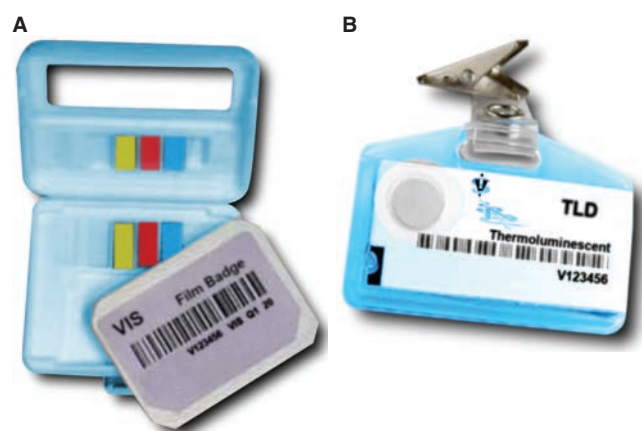
Figure 1.70 Types of dosimetry. Pictured are a film Badge (A) and a Thermoluminescent dosimeter (B). The plastic badge is propped open with the envelope containing the film sitting outside it. The series of filters is visible.
