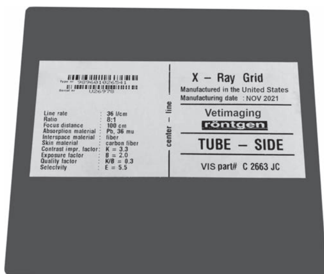
Figure 1.40 Grid. A picture of the front of a grid depicting a typical label that lists the characteristics of the grid including type, composition, ratio, frequency, focal distance, and others.
