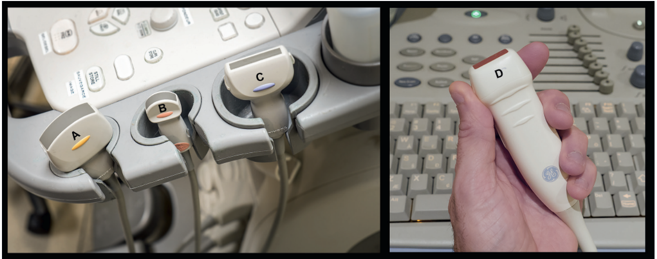
Figure 1.4. Practical ultrasound transducers. Most ultrasound units are equipped with convex (A, B) and linear (C) electronic transducers with variable frequencies. A macroconvex probe offering lower frequencies (3–8 MHz) is best suited for the abdomen of large dogs, whereas a microconvex probe (B) of higher frequency and smaller footprint is preferred for the abdomen of small patients and when only a small acoustic window is available (e.g., intercostal approach of a lung lesion). A high-frequency (10–18 MHz) linear probe is most useful for assessing superficial structures on a relatively wide and flat surface (e.g., assessing bowels in a cat, biceps tendon in a dog). A phased array transducer (D) offers a small flat footprint and is ideal for echocardiography.
